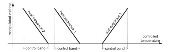
Fig 5 [Coils control - Assign a control sequence to a coil 01]
