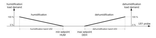
Fig 49 [Humidity control - Control sequences]
