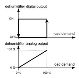
Fig 51 [Humidity control - Dehumidifier control]
