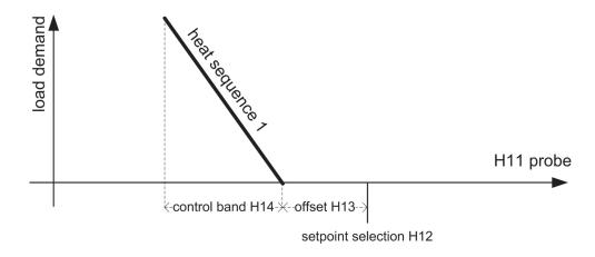
Fig 27 [Temperature control sequences - Heat control sequences 1]
