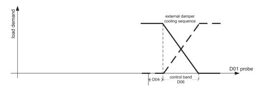
Fig 19 [Temperature control sequences - d00=DCS]
