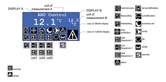
Fig 2 [User interface - LCD display]
