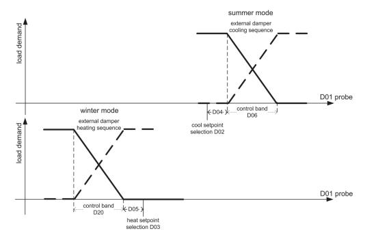
Fig 21 [Temperature control sequences - d00=AUTO]
