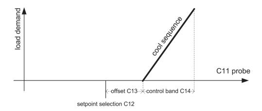
Fig 29 [Temperature control sequences - Cool sequences]
