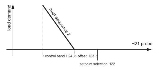
Fig 28 [Temperature control sequences - Heat control sequences 2]
