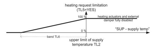
Fig 47 [Controlling the supply temperature limits - Supply temperature upper limit]
