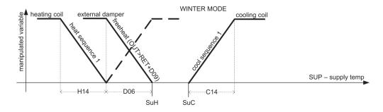
Fig 41 [Examples - Dampers, heating coil and cooling coil 2]
