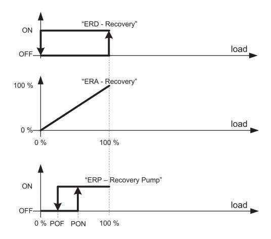
Fig 18 [Dampers and energy recovery control - Energy recovery]
