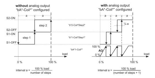
Fig 8 [Coils control - Linear step switch]
