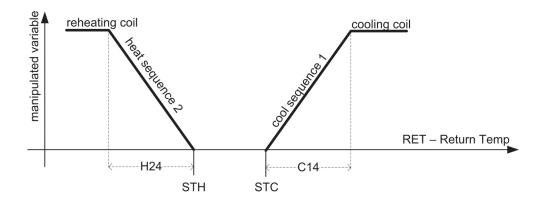
Fig 38 [Examples - Cooling and reheating coil]
