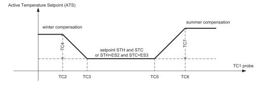
Fig 31 [Temperature control sequences - Temperature compensation]
