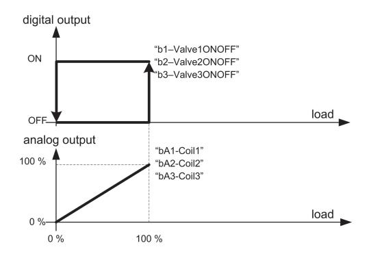
Fig 7 [Coils control - ON/OFF and 0/10 V valve control]
