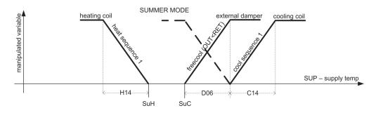
Fig 42 [Examples - Dampers, heating coil and cooling coil 3]
