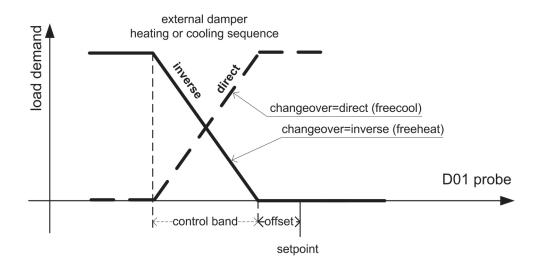
Fig 22 [Temperature control sequences - D21, D23=CHP]
