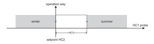
Fig 13 [Coils control - Heat/cool selection]
