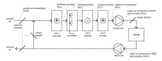
Fig 4 [Configuring the AHU software - Configuration overview]
