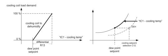
Fig 54 [Humidity control - Cooling coil in dehumidification 3]
