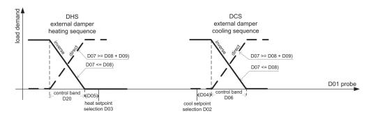
Fig 25 [Temperature control sequences - Changeover condition]
