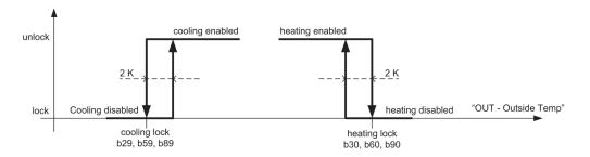
Fig 11 [Coils control - Locking sequences]
