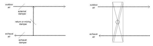
Fig 15 [Dampers and energy recovery control - Damper sequence]
