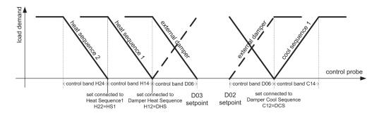
Fig 30 [Temperature control sequences - Connection of setpoint sequences]
