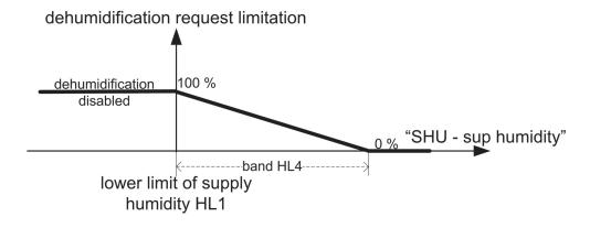
Fig 57 [Humidity control - Lower limit]
