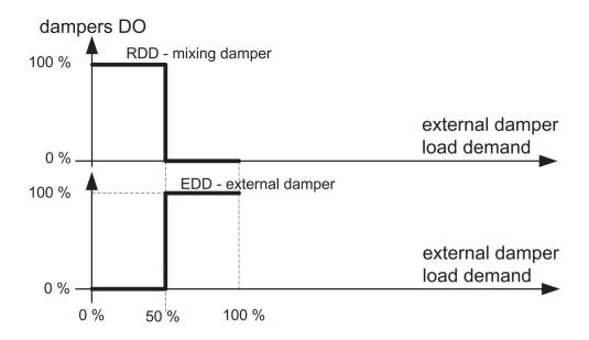
Fig 16 [Dampers and energy recovery control - ON/OFF dampers]
