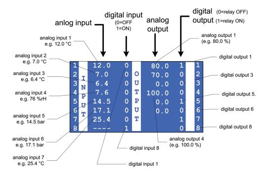
Fig 3 [User interface - Input/output values - LCD display]
