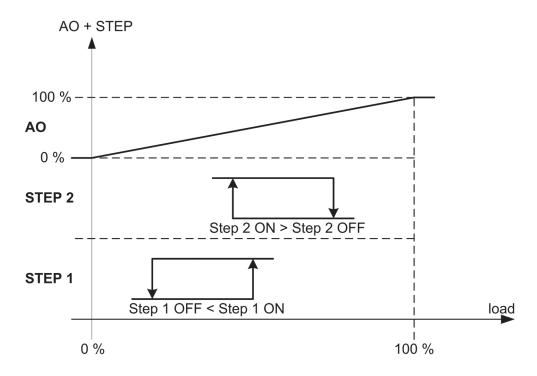
Fig 9 [Coils control - Variable step switch]
