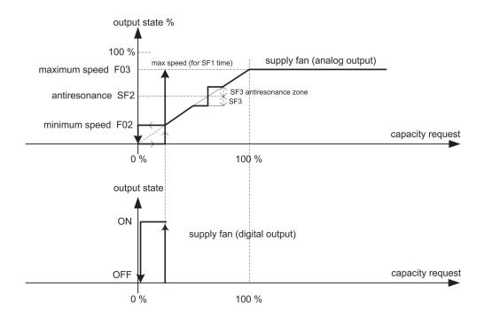
Fig 59 [Supply and return fans - Fan speed configuration]
