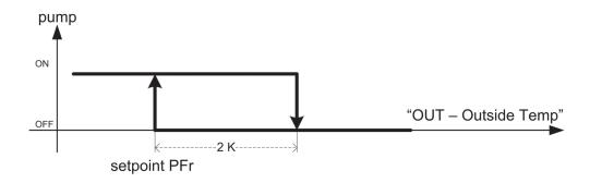
Fig 12 [Coils control - Pumps winter start]
