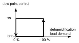
Fig 53 [Humidity control - Cooling coil in dehumidification 2]
