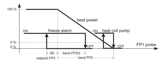
Fig 43 [Frost protection - Alarm setpoint FP2]
