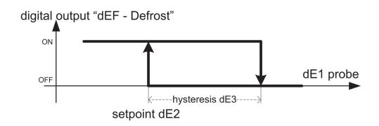
Fig 14 [Coils control - Cooling coil defrost control]
