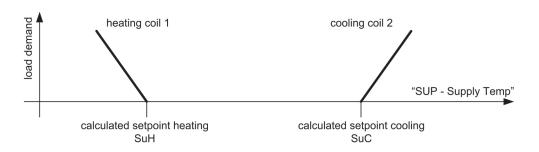
Fig 35 [Cascade control - Setpoint]
