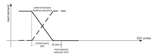
Fig 20 [Temperature control sequences - d00=DHS]
