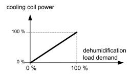
Fig 55 [Humidity control - Cooling coil in dehumidification 4]
