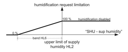
Fig 56 [Humidity control - Upper limit]
