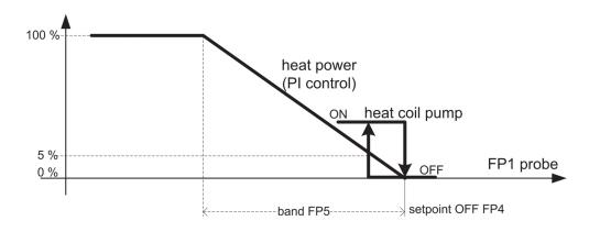
Fig 44 [Frost protection - Frost prevention in OFF]
