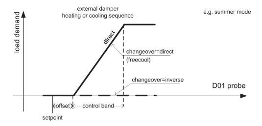
Fig 24 [Temperature control sequences - D21, D23=DIR]
