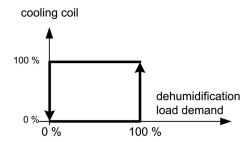
Fig 52 [Humidity control - Cooling coil in dehumidification]
