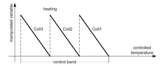
Fig 6 [Coils control - Assign a control sequence to a coil 02]
