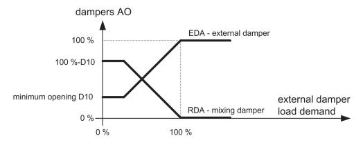
Fig 17 [Dampers and energy recovery control - 0/10 V dampers]
